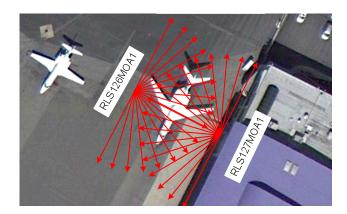
The lines in red designate the coverage area of the Optex RLS-3060. If an intrusion occurs in the coverage area as detected by the Optex RLS-3060, the alarming unit will then send a TCP or UDP ASCII string to the Milestone VMS (Video Management Software) system.
